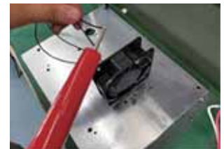
Step 8. Test high voltage
